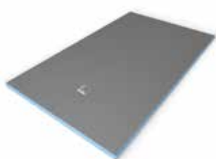
01 wedi Fundo Primo The original wedi Fundo: Robust, pre sloped, waterproof, shower floor bases with 4"x 4" drain cover. Customizable on site. Often installed on substrates and used with wedi curbs.
